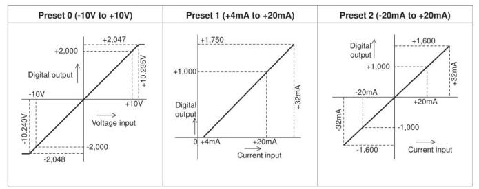
**NOTE:** Preset ranges are selected by an appropriate setting in buffer memory of the analog block.Current/Voltage input selection must match the correct input terminal connections.
